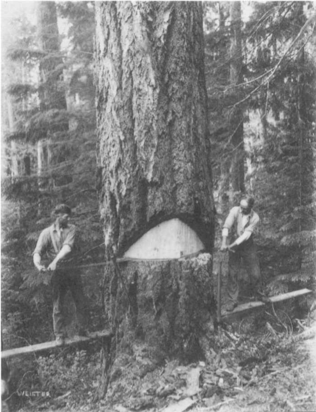
Standing on springboards to provide a level work platform above the brush on steep ground, two loggers in the 1920s begin falling a Douglas fir. Note the kerosene bottles (for cutting the pitch buildup on the sawblade) below saw to the left and above to the right and the two doublebitted axes with which the fallers will make an undercut (indicated by the area stripped of bark) that will bring the tree down.
