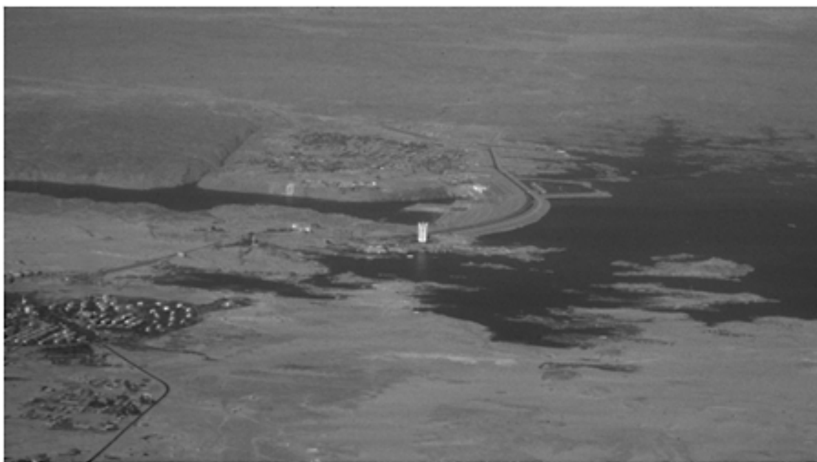
Figure 7.5 Aerial view of the Aswan High Dam on the Nile River in Egypt; Lake Nasser to the right. This dam, which ended the annual flooding of the Nile below it, impounds two years' flow of the river. It has been hailed as one of the greatest projects of the twentieth century and denounced as a major ecological catastrophe. Photograph taken in 1981.
