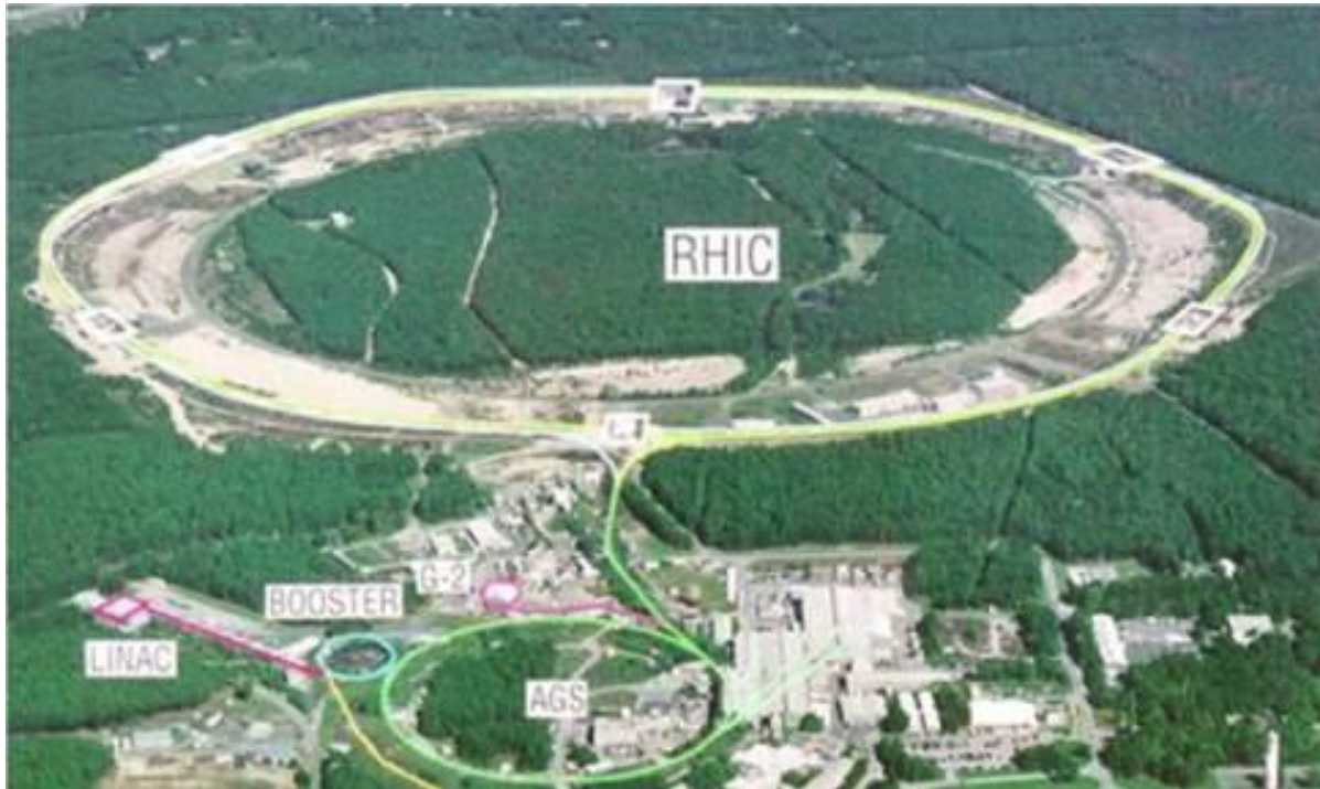
Figure 8: The Relativistic Heavy Ion Collider (RHIC) complex at Brookhaven National Laboratory (BNL). The circumference of its ring is 3900 meters. Gold ions are produced in a Tandem Van de Graaff (not shown) and sent via a transfer line to a Booster to increase their energy. From there they are sent to the AGS (Alternating Gradient Synchrotron) where their energy is increased further. Finally they are sent to RHIC, half going in a clockwise direction and half going in a counter-clockwise direction, and accelerated to their final energy. The LINAC (Linear Accelerator) produces protons for use in the AGS and RHIC. Credit: Courtesy of Brookhaven National Laboratory.
