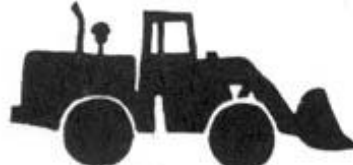
Articulated Loader (pivots in center)
