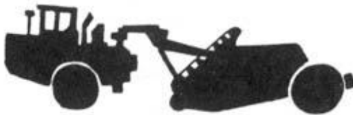
Scraper (w/2-wheeled tractor)
