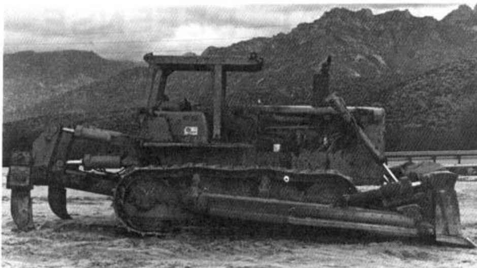
Bulldozer. Note the smoke stack (exhaust pipe).
